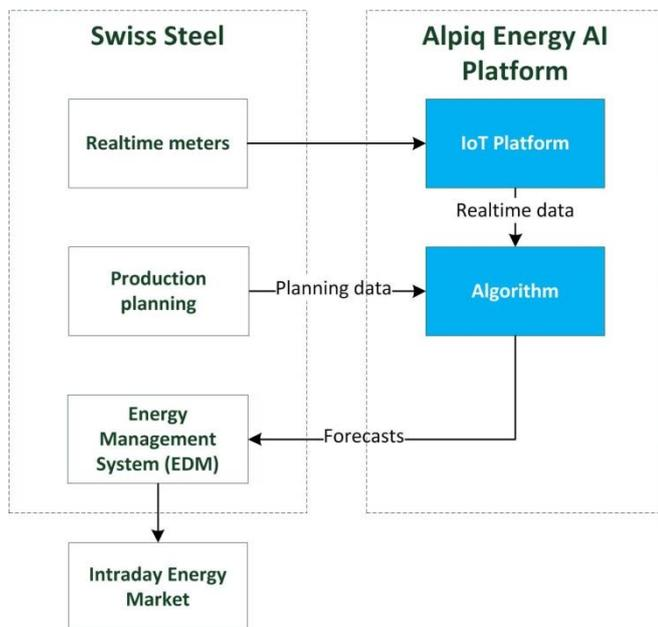
Figure 1: Illustration of the technical setup for the Energy AI real-time forecasting.
